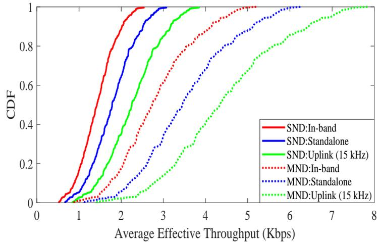
Fig. 1. Average effective throughput in different deployment scenarios with both SND and MND
